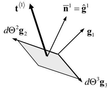
**Figure 3.10.2: traction acting on a surface element**
