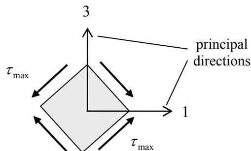
**Figure 3.4.3: maximum shear stress at a point**
