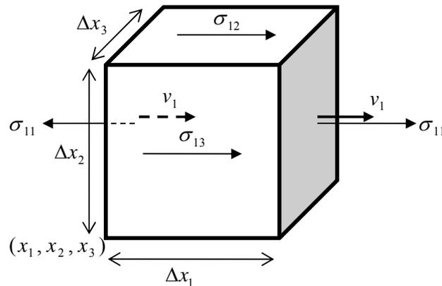
**Figure 3.8.1: A differential mass element subjected to stresses**
