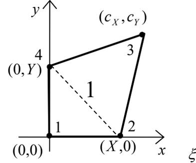
The Jacobian can be zero or negative for certain values of  $\xi$  and  $\eta$ , for certain values of  $c_X, c_Y$ . For example, although it is positive at nodes 1, 2 and 4, at node 3 it is negative for
