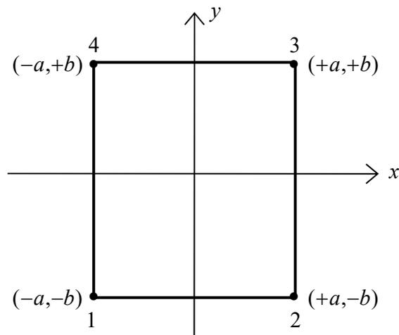
$$\begin{aligned} N_1(x, y) &= \frac{1}{4ab}(a-x)(b-y) \\ N_2(x, y) &= \frac{1}{4ab}(a+x)(b-y) \\ N_3(x, y) &= \frac{1}{4ab}(a+x)(b+y) \\ N_4(x, y) &= \frac{1}{4ab}(a-x)(b+y) \end{aligned} \quad (6.1)$$
