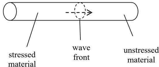
**Figure 4.9: wave propagation along an elastic rod**
