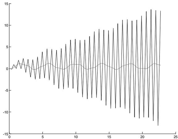
**Figure 4.13: unstable displacement solution**
