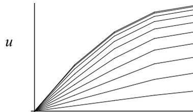
**Figure 4.11: deformed shapes of the elastic bar (Note: this picture gives the impression that the bar is swaying up and down (like a beam); actually, these displacements are along the direction of the rod – it is all one-dimensional)**
